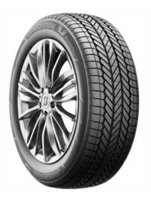
225/55R19 99V Bridgestone WeatherPeak BW Part Number: 009642 Load Index: 99 Speed Symbol: V Sidewall: BW Treadwear: 700 Traction: A Temperature: A Tread Depth: 10 Approved Rim Width: 6 - 8 Section Width In: 9.20 Overall Diameter: 28.80 Max Load (Single): 1709 Tread Expectancy: 70000 Weight: 25.91 Road Hazard: N
